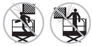
Be aware of crushing hazards when grasping the platform guard rail.
